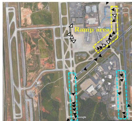
Fig. 1. Airport layout for Charlotte Douglas International airport (CLT). The flights taxiing-in and those taxiing-out are represented by gray and black triangles, respectively. The ramp queue and runway queue are shown in yellow and cyan, respectively.
