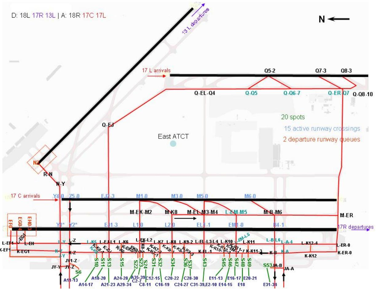
Figure 3. Node-link model of Eastern half of DFW in A 17LC, 18R, 13R/D 17R, 13L, 18L configuration, showing the taxiways, runways and intersections. The intersection labels those used by the SMS adaptation for DFW.
