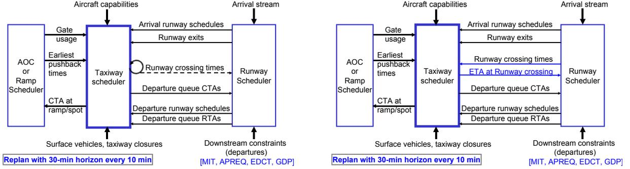
Figure 1. (Left) Optimization architecture diagram, showing interactions between ramp, taxiway and runway schedulers. (Right) Potential modification of interaction between runway and taxiway schedulers.
