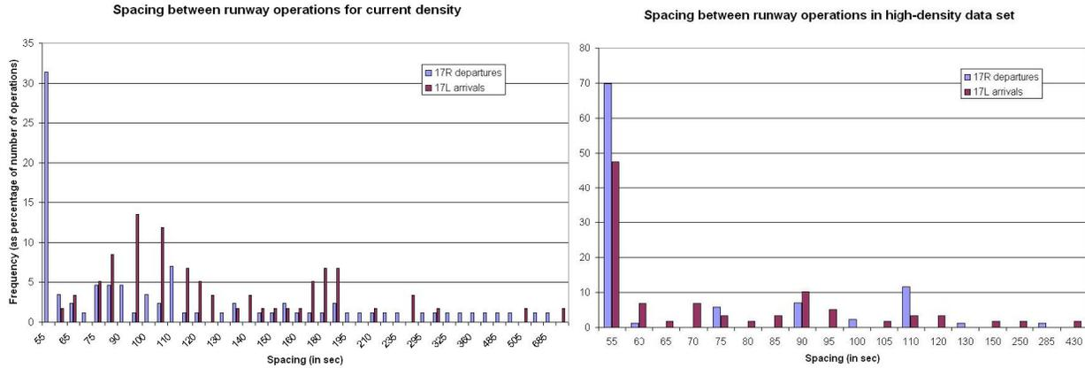
Figure 5. Histogram of inter-arrival and inter-departure spacings for current operations (left) and the high-density data set (right). Note that the scales are not the same.
