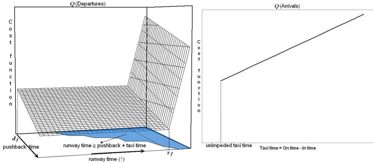
Figure 4. [Left] Form of objective function,  $Q(\text{Departures})$ . The shaded region denotes the feasible set of pushback and runway times. [Right] Cost function for arriving aircraft,  $Q(\text{Arrivals})$
