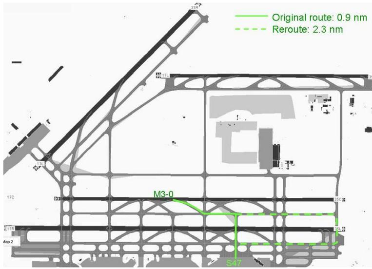
Figure 6. An example of a taxi reroute from runway exit M3-0 to Spot 47 (Gate 16). The original route is 0.9 nm long, while the alternate route is 2.3 nm long.
