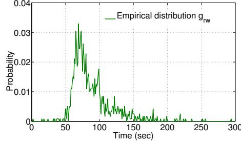
**Figure 2.** Empirical service time probability distribution for departures of 22L, 27 | 22L, 22R at BOS.
