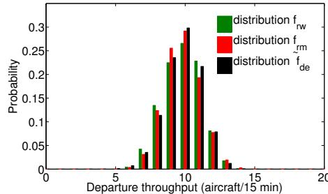
**Figure 4.** Empirical departure throughput distribution,  $f_{rw}$ , and fits  $f_{rm}$  and  $\tilde{f}_{de}$  for 22L, 27 | 22L, 22R at BOS.
